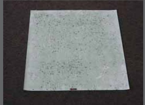
PVC membrane with a lacquer-coated top ply
